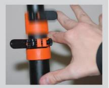
If the clamp does detach from the section, it can easily be glued back in place using a 2-part adhesive (available from lonic or from most hardware stores).
