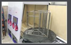
After a full and detailed examination, the chassis is stripped of all of the components and the tank is removed for flushing. The steel frame is cleaned and then the abrasive blasting treats the stainless steel surface. At this point, the refurbished machine chassis is indistinguishable from a newly manufactured one.
