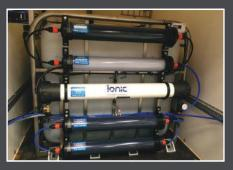
The chassis is then re-united with the cleaned and pressure-tested tank, and any new components are mounted. The refurbished machine is then subjected to exactly the same testing procedure as a brand new system.
